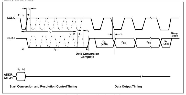
Figure 2. Conversion and Data Output Timing
