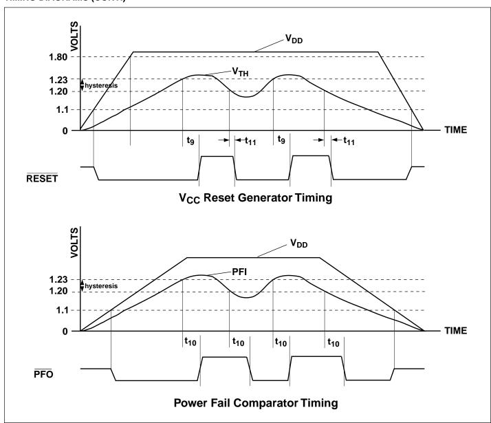
Figure 5. Reset and Power Fail Timing
