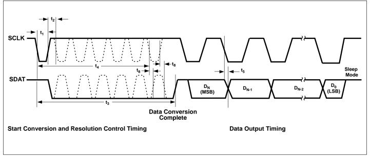
Figure 2. Conversion and Data Output Timing
