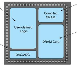
The megacell compiler software can generate a wide range of high-density SRAMs and ROMs in low-power models.
