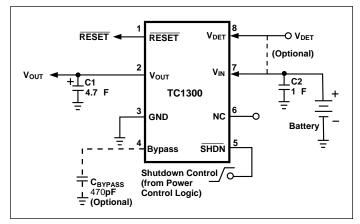
Figure 1: Typical Application Circuit
