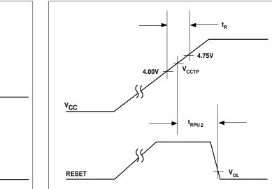
Figure 3. Timing Diagram: Power Up (TC1274)
