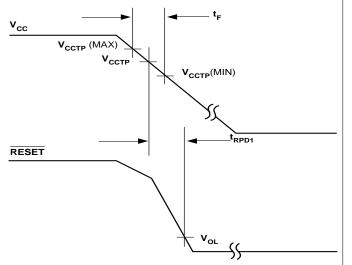
Figure 2. Timing Diagram: Power Down (TC1272, TC1273)
