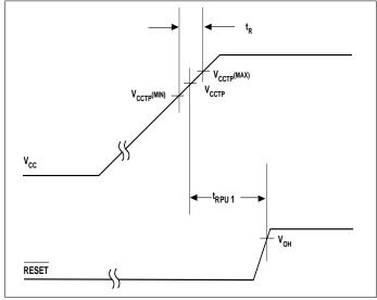
Figure 1. Timing Diagram: Power Up (TC1272, TC1273)
