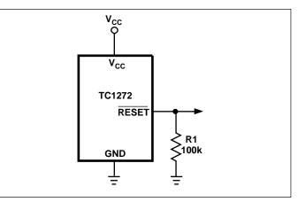
Figure 6. Ensuring RESET Valid to  $V_{CC} = 0V$
