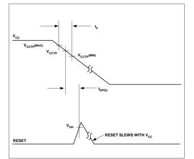
Figure 4. Timing Diagram: Power Down (TC1274)
