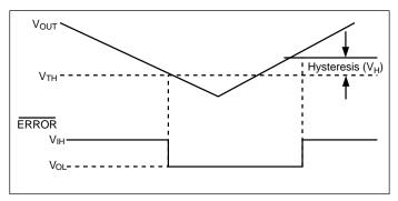
Figure 3: ERROR Output Operation
