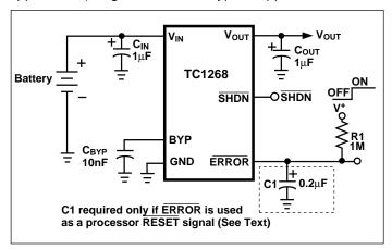
Figure 1: Typical Application Circuit
