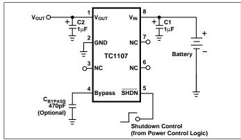
Figure 1. Typical Application Circuit
