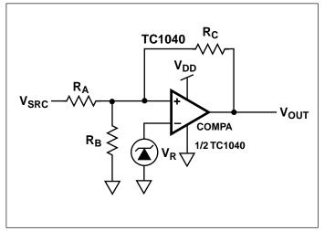
Figure 3.Comparator External Hysteresis Configuration
