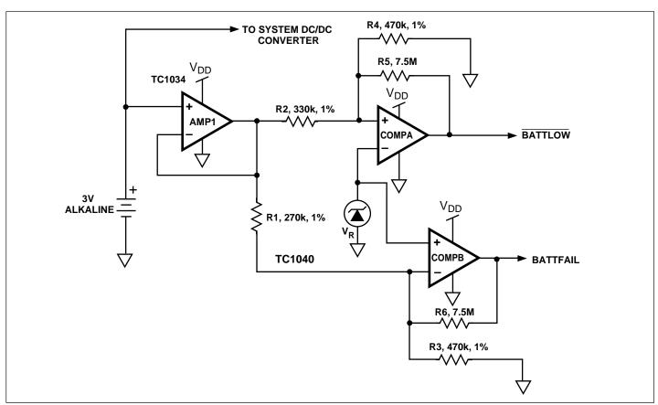
Figure 2. Precision Battery Monitor
