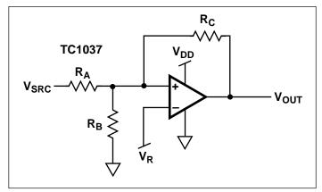
Figure 1. Comparator External Hysteresis Configuration
