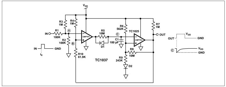
Figure 4. Non-Retriggerable Multivibrator
