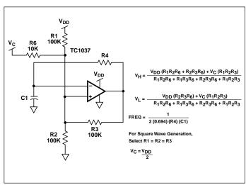
Figure 6. Pulse Width Modulator
