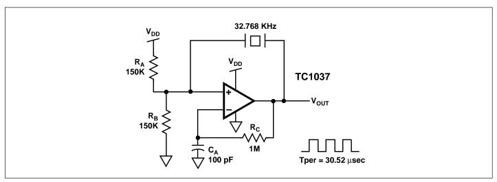
Figure 3. 32.768 KHz "Time of Day" Clock Oscillator
