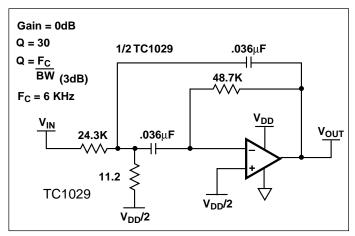
Figure 2. Second Order SAT Bandpass Filter
