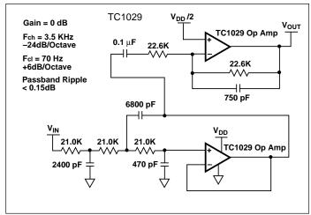
Figure 1. Multi-Pole Butterworth Voice Band Receive Filter
