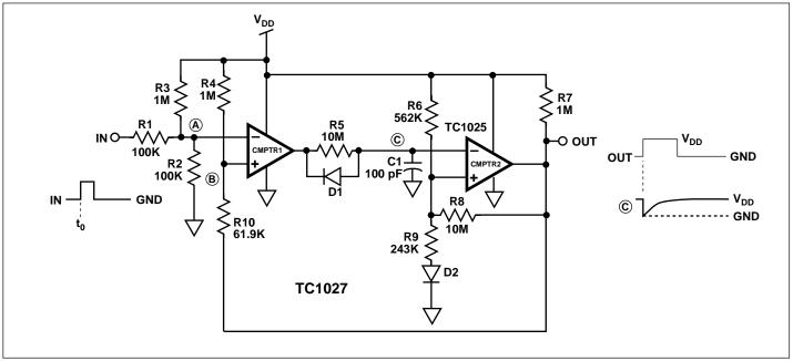
Figure 4. Non-Retriggerable Multivibrator
