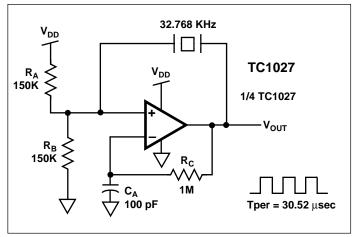
Figure 3. 32.768 KHz "Time of Day" Clock Oscillator
