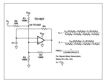
Figure 6. Pulse Width Modulator
