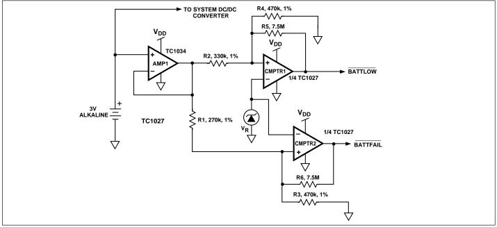
Figure 2. Precision Battery Monitor
