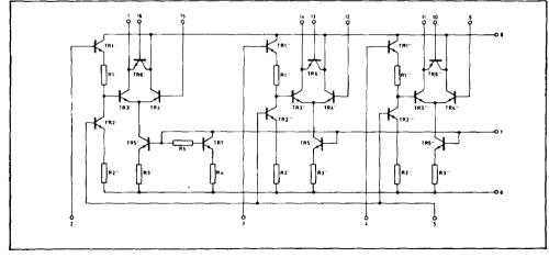
Fig. 2 TBA530 block diagram
