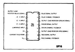
Fig. 1 Pin connections
