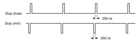
The voltage applied to the motor is duty 100% because of the storage time of the drive circuit even if the duty is 99%.
