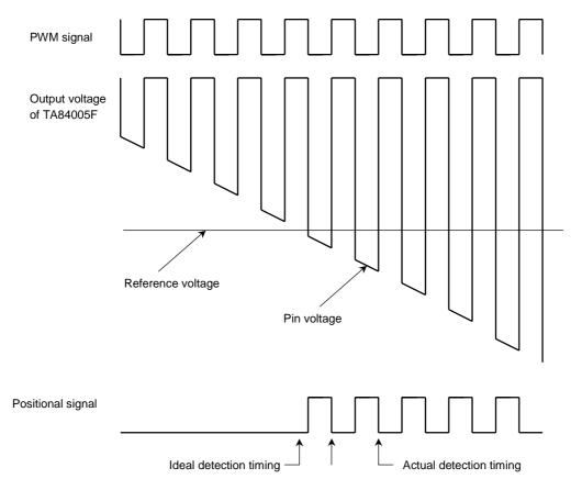
$\label{eq:Variation} \begin{array}{ll} \mbox{Variation is calculated by detecting at two consecutive rising edges of PWM signal.} \\ 1/f_p < \mbox{Detection time variation} < 2/f_p & f_p \mbox{: PWM frequency} \end{array}$
