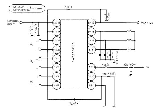
Note: Utmost care is necessary in the design of the output line, V<sub>CC</sub> and GND line since IC may be destroyed due to short-circuit between outputs, air contamination fault, or fault by improper grounding.
