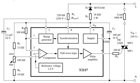
Figure 1. Block diagram with typical circuit, period group control 0 to 100%
