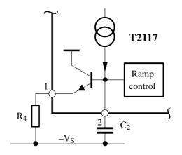
Figure 3. Pin 1 internal network
