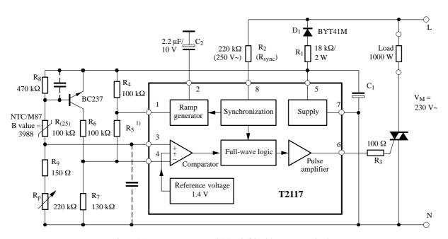
Figure 11. Temperature control 15 to 35°C with sensor monitoring
