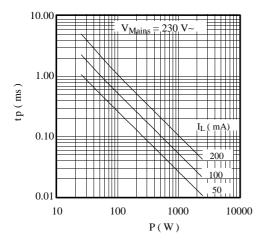
Figure 5. Output pulse width
