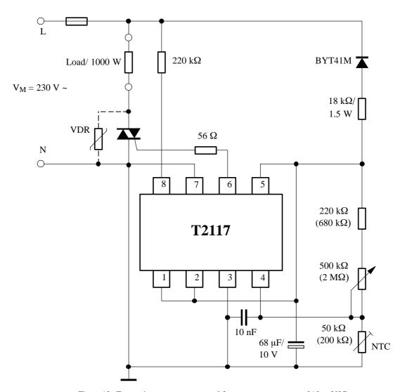
Figure 13. Two–point temperature control for a temperature range of 15 to  $30^{\circ}\mathrm{C}$
