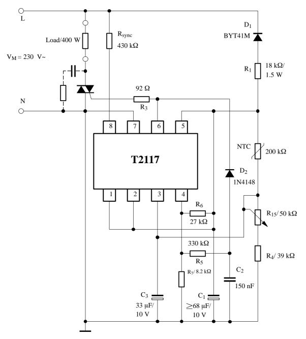
Figure 14. Two-point temperature control for a temperature range of 18 to 32°C and a hysteresis of  $\pm 0.5$ °C at 25°C
