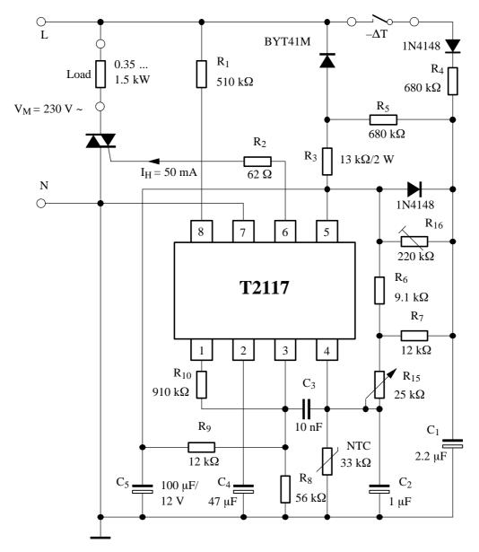
Figure 12. Room temperature control with definite reduction (remote control) for a temperature range of 5 to  $30^{\circ}$ C
