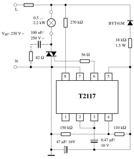
Figure 9. Power blinking switch with f  $\approx$  2.7 Hz, duty cycle 1:1, power range 0.5 to 2.2 kW
