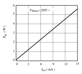
Figure 8. Power dissipation of R<sub>1</sub> according to current consumption
