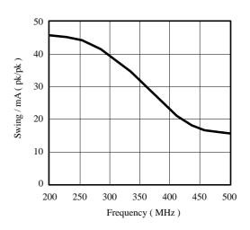
Figure 5. Frequency dependency of swing (RS =  $680 \Omega$ )
