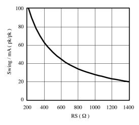
Figure 4. Swing vs. resistor RS (RF =  $6.8 \text{ k}\Omega$ )
