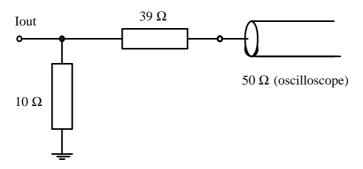
Figure 6. Test circuit for measurement of write rise and fall time
