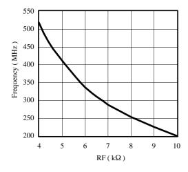
Figure 3. Frequency vs. resistor RF (RS =  $680 \Omega$ )
