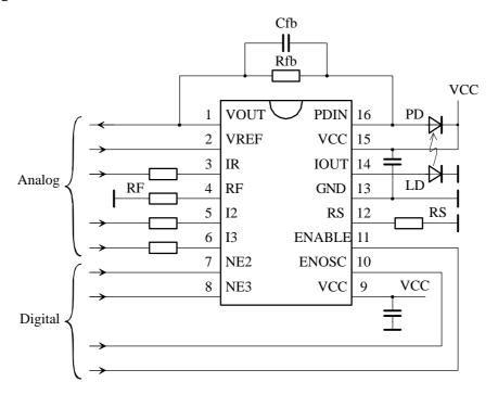
Figure 8. Application circuit
