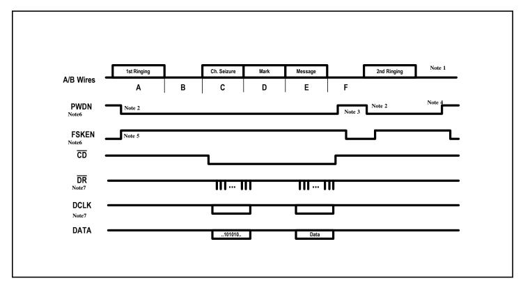
Figure 11. Bellcore On-hook Data Transmission Timing Diagram
