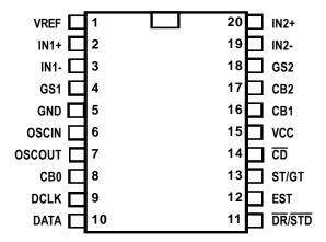
Figure 2. Pin Assignment
