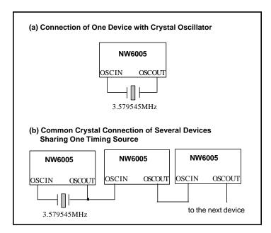
Figure 8. Application of Clock Driven Circuit
