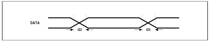
Figure 19. DATA Output Timing in Mode '0'
