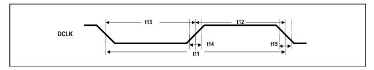
Figure 17. DCLK Timing in Mode '1'
