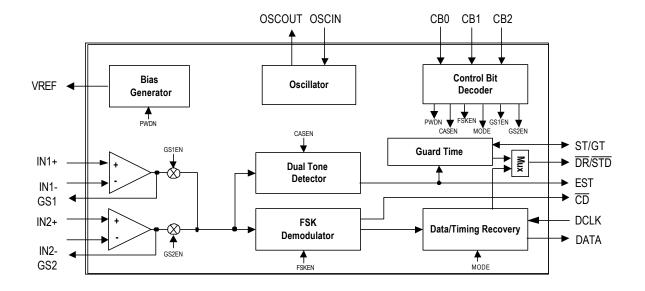
Figure 1. Block Diagram
