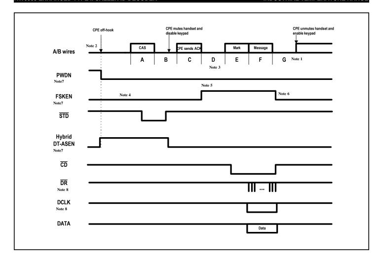
Figure 12. Bellcore Off-hook Data Transmission Timing Diagram
