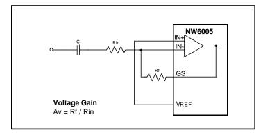
Figure 4. Single-ended Input Gain Control Circuit
