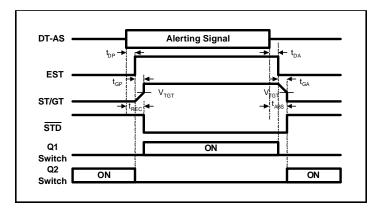
Figure 6. Guard Time Waveform
