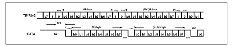
Figure 20. Serial Data Interface Timing in MODE '0'
