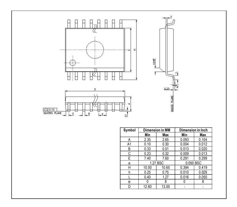
Figure 21. NW6005-XS 20 Pin SOIC Package Diagram
