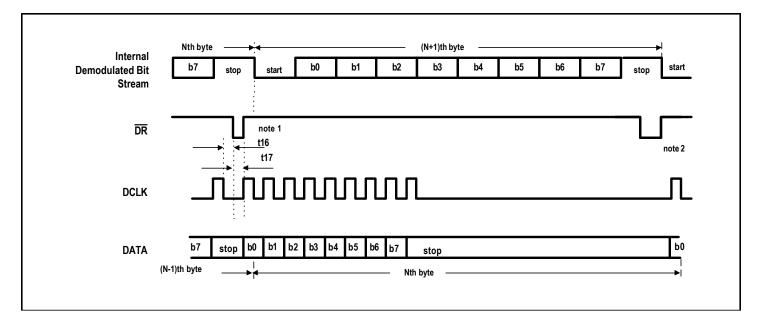
Figure 18. Serial Data Interface Timing in MODE '1'
