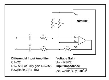
Figure 3. Differential Input Gain Control Circuit
