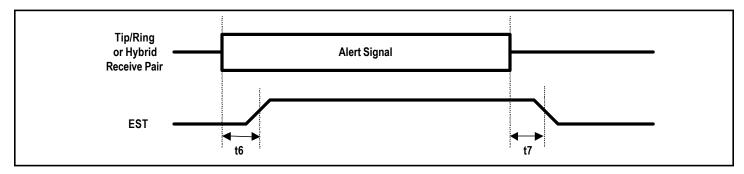
Figure 16. Dual Tone Alert Signal Detection Time
