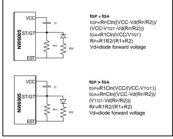
Figure 7. Guard Time Circuits with Unequal Present and Absent Times
