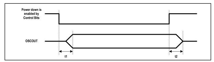
Figure 14. Power Up/Down Timing
