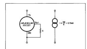
Figure 5. A Two-Component Precision Current Limiter
