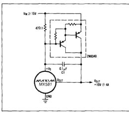
Figure 3. High Current Precision Supply
