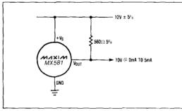
Figure 4. 12-Volt Supply Connection
