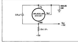
Figure 6. Two-Terminal –10 Volt Reference
