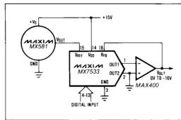
Figure 7. Low Power 10 Bit CMOS DAC Connection
