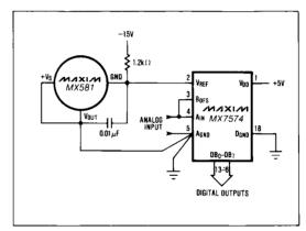
Figure 8. Negative 10V Reference for CMOS A/D Converter
