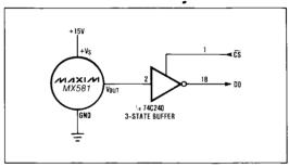
Figure 9. MX581 Microprocessor Interface
