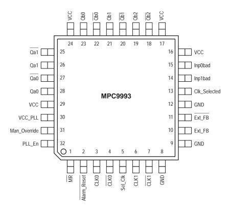
Figure 2. 32-Lead Pinout (Top View)
