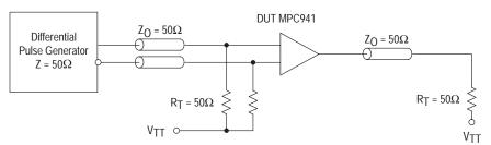
Figure 13. PECL\_CLK MPC941 AC test reference for  $V_{CC}$  = 3.3V and  $V_{CC}$  = 2.5V
