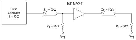
Figure 12. LVCMOS\_CLK MPC941 AC test reference for V<sub>CC</sub> = 3.3V and V<sub>CC</sub> = 2.5V
