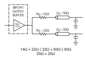
Figure 3. Optimized Dual Line Termination
