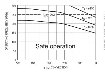
Figure 6. Maximum MPC941 frequency, V<sub>CC</sub> = 3.3V, MTBF 4 years, driving series terminated transmission lines
