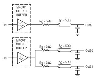
Figure 1. Single versus Dual Transmission Lines
