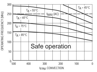
Figure 7. Maximum MPC941 frequency, V<sub>CC</sub> = 3.3V, MTBF 4 years, 4 pF load per line
