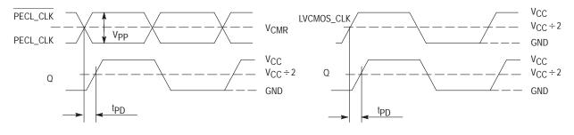
Figure 14. LVPECL Propagation delay (tpp) test reference
