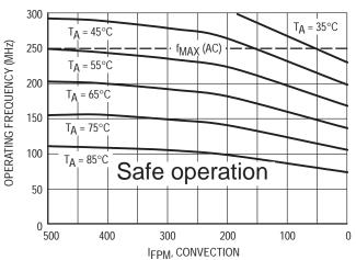
Figure 5. Maximum MPC941 frequency, V<sub>CC</sub> = 3.3V, MTBF 9.1 years, 4 pF load per line
