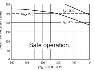
Figure 11. Maximum MPC941 frequency, V<sub>CC</sub> = 2.5V, MTBF 4 years, 4 pF load per line
