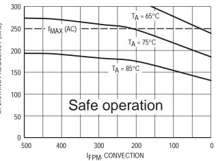
Figure 9. Maximum MPC941 frequency, V<sub>CC</sub> = 2.5V, MTBF 9.1 years, 4 pF load per line
