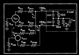
FIGURE 2. MPC800 Static Accuracy Equavalent Circuit (Differential Operation).
