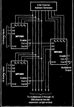
FIGURE 6. Channel Expansion up to 256 Channels Using 16 X 16 Two-tiered Expansion.
