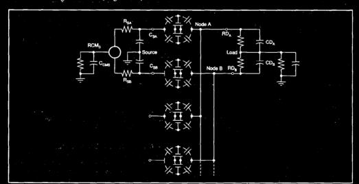
FIGURE 4. Settling and Common-Mode Effects (Differential).
