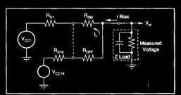
FIGURE 1. MPC800 Static Accuracy Equavalent Circuit (Single-ended Operation).
