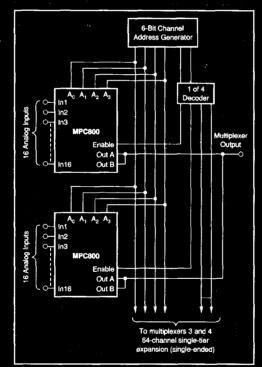
FIGURE 5. 32- to 64-Channel, Single-tier Expansion.
