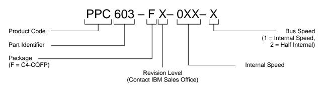
Figure 18. IBM Part Number Key
