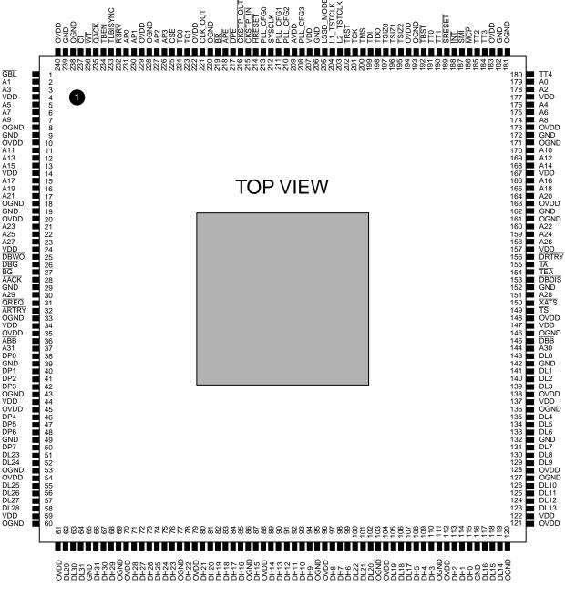
Figure 9. Pinout Diagram of the CQFP Package
