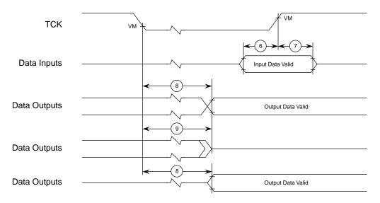
Figure 7. Boundary-Scan Timing Diagram
