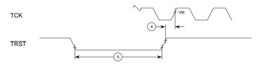
Figure 6. TRST Timing Diagram
