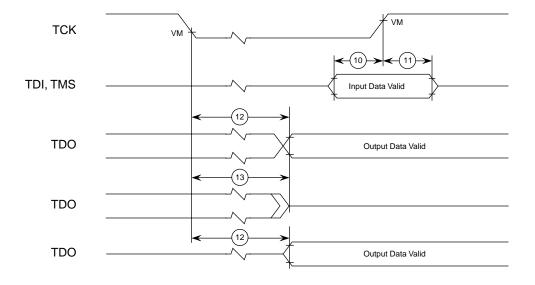
Figure 8. Test Access Port Timing Diagram
