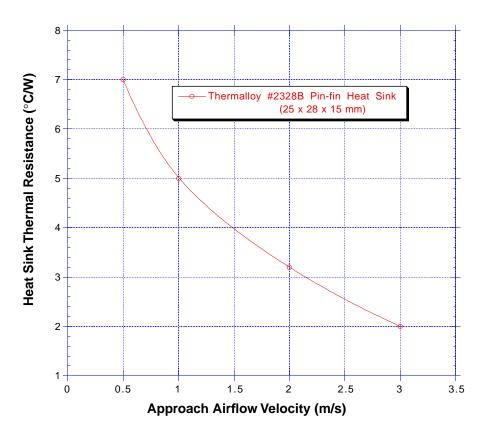
Figure 16. Thermalloy #2328B Heat Sink-to-Ambient Thermal Resistance Versus Airflow Velocity
