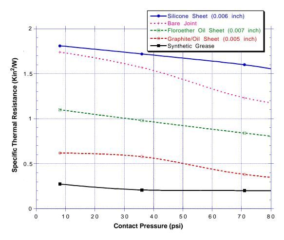
Figure 15. Thermal Performance of Select Thermal Interface Material
