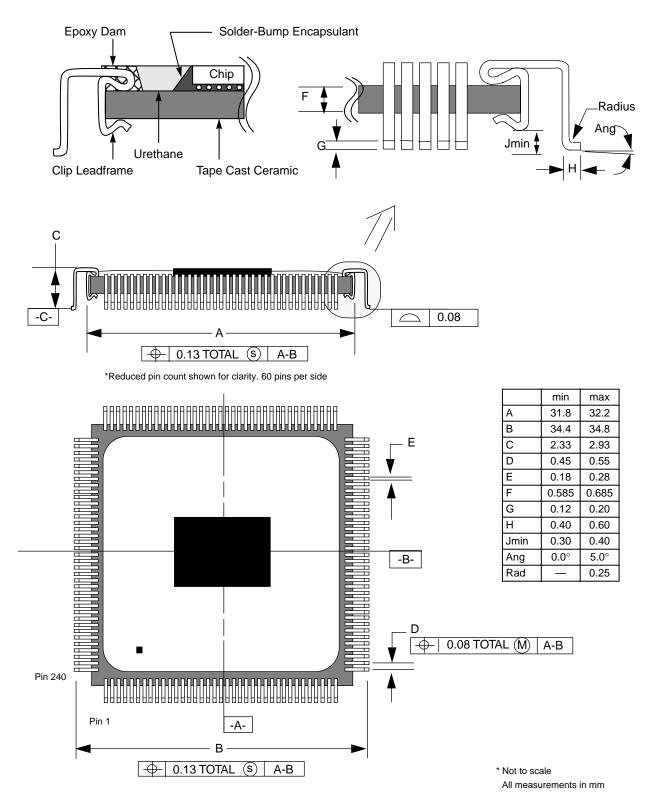
Figure 11. Mechanical Dimensions of the IBM C4-CQFP Package
