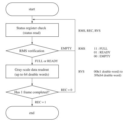
• Gray-scale data readout processing flowchart description This operation reads out the gray-scale data created by the IC.
