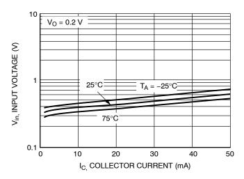
Figure 6. Input Voltage vs. Output Current
