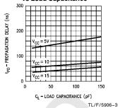
MM54C373/MM74C373, MM54C374/MM74C374 Change in Propagation Delay per pF of Load Capacitance ( $\Delta t_{PD}/pF$ ) vs Power Supply Voltage
