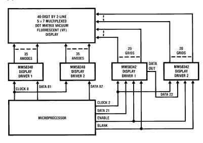
FIGURE 6. Microprocessor-Controlled Word Processor
