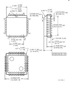
Plastic Chip Carrier (V) Order Number MM58342V NS Package Number V28A
