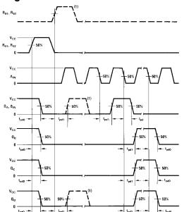
Note 1: MM54C90, MM74C90 and MM54C93, MM74C93 are solid line waveforms. Dashed line waveforms are for MM54C90/MM74C90 only.
