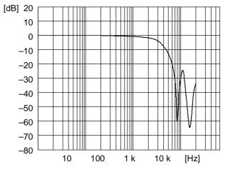
Figure 10.1 LPF Frequency Characteristics (f<sub>SAM</sub> = 8 kHz)
