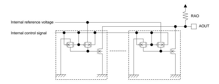
As shown above, the ML2215 uses current type DACs.
