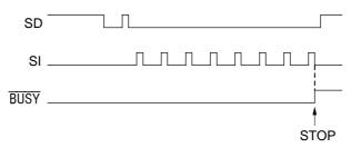
Figure 6.1 Timing for Stop Code Input - 2-pin Interfacing
