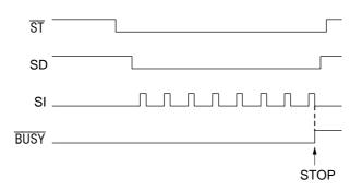
Figure 6.2 Timing for Stop Code Input - 3-pin Interfacing
