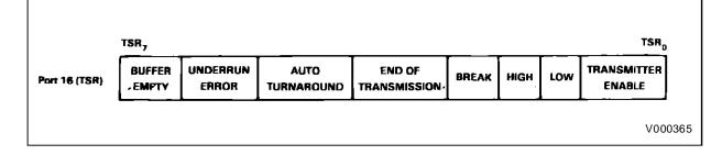
Figure 19: Transmitter Status Register (TSR).
