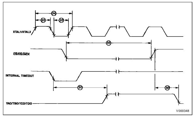
Figure 30 : Reset Timing.
