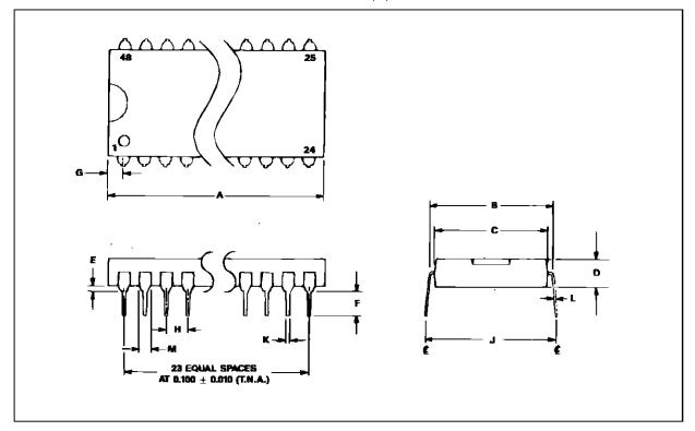
MK68901 48-PIN PLASTIC DUAL-IN-LINE PACKAGE (N)
