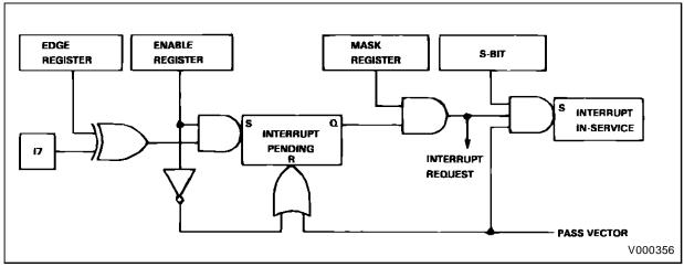
Figure 10: A Conceptual Circuit of an Interrupt Channel.
