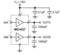
Figure 2a. Noninverting Configuration
