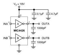
Figure 1a. Inverting Configuration
