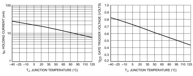
Figure 5. Typical Holding Current versus Junction Temperature
