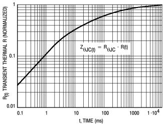
Figure 4. Transient Thermal Response
