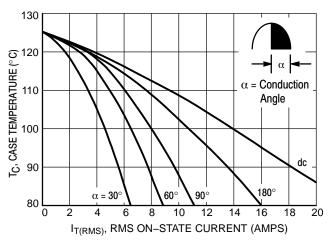
Figure 7. Typical RMS Current Derating
