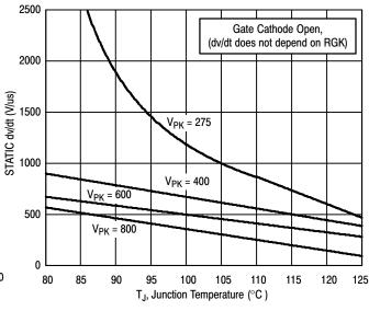
Figure 10. Typical Exponential Static dv/dt Versus Junction Temperature
