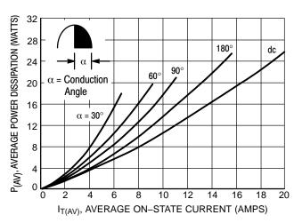
Figure 8. On State Power Dissipation
