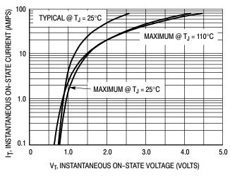
Figure 3. On-State Characteristics
