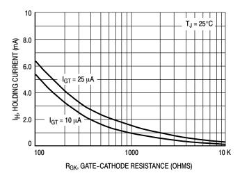
Figure 9. Holding Current versus Gate-Cathode Resistance
