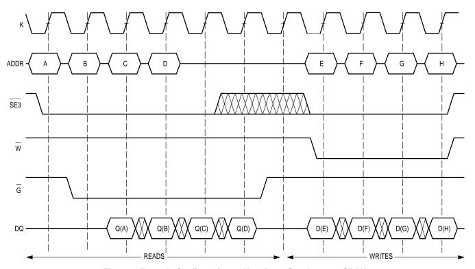
Figure 2. Example Configuration as Non-Burst Synchronous SRAM
