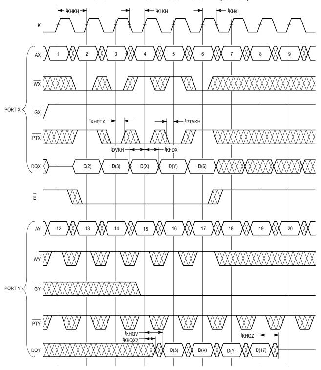
$\overline{E}$  Low =  $\overline{E1}$  Low and E2 High.  $\overline{E}$  High =  $\overline{E1}$  High or E2 Low.
