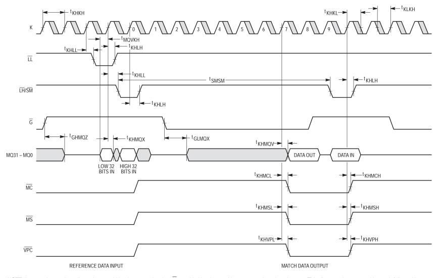
NOTE: In normal operation, all matches would be the same size, i.e., LL would either be used in every match cycle or in none. This diagram shows a 64-bit match followed by a 32-bit match in order to illustrate all the key specs.
