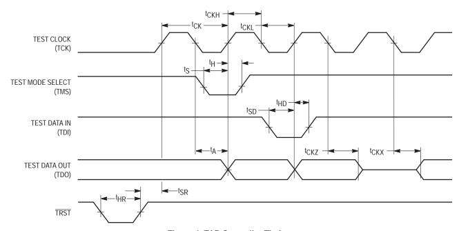
Figure 4. TAP Controller Timing
