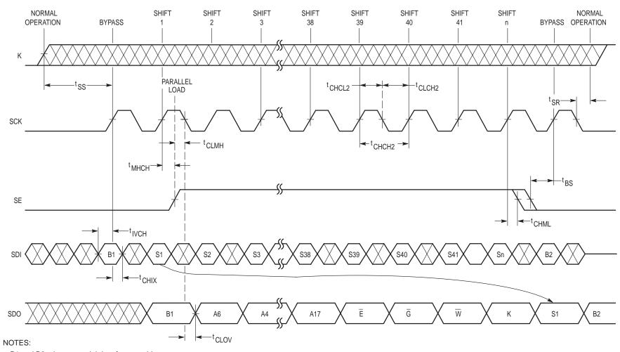
B1 and B2 = bypass serial data from outside source.
