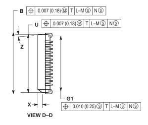
NOTES: 1. DATUMS –L-, –M-, AND –N– DETERMINED WHERE TOP OF LEAD SHOULDER EXITS PLASTIC BODY AT MOLD PARTING LINE. ⊕ 0.007 (0.18) M T L-M S N S 2. DIMENSION G1, TRUE POSITION TO BE MEASURED AT DATUM -T-, SEATING PLANE. 3. DIMENSIONS R AND U DO NOT INCLUDE MOLD 0.007 (0.18) M T L-M S NS
