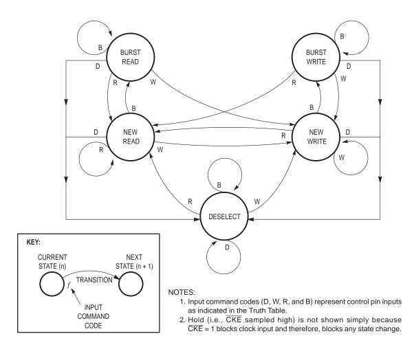
Figure 1. ZBT RAM State Diagram
