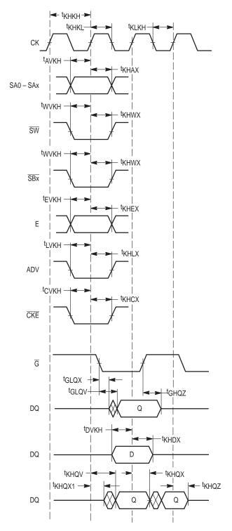
**Figure 7. AC Timing Parameter Definitions**
