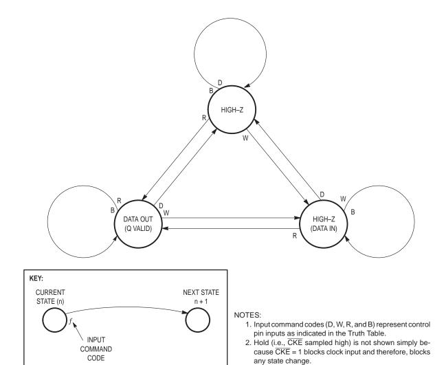
Figure 3. Data I/O State Diagram
