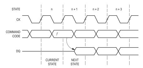
Figure 2. State Definitions for ZBT RAM State Diagram
