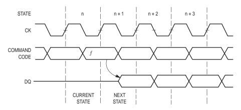
Figure 4. State Definitions for ZBT RAM State Diagram
