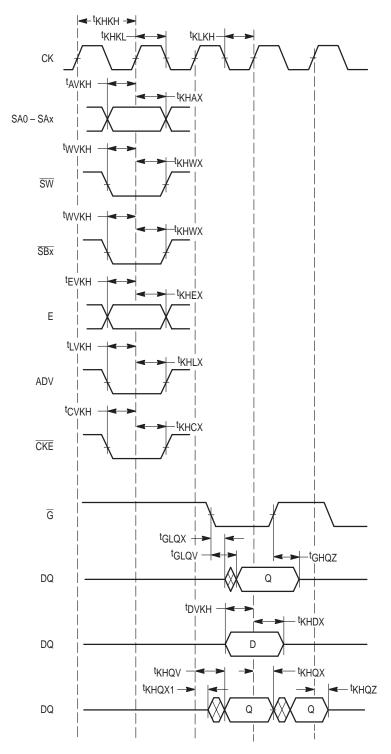
Figure 7. AC Timing Parameter Definitions
