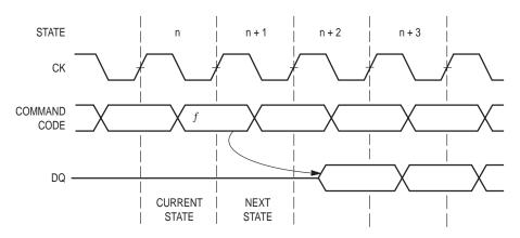
Figure 2. State Definitions for ZBT RAM State Diagram
