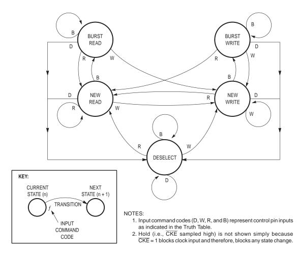
Figure 1. ZBT RAM State Diagram
