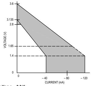
(b) Pull-Up:  $V_{DDQ} = 3.3 V$
