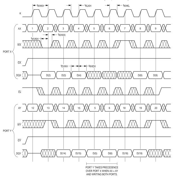
NOTE:  $\overline{Ex}$  Low =  $\overline{E1x}$  Low and E2x High.  $\overline{Ex}$  High =  $\overline{E1x}$  High or E2x Low.
