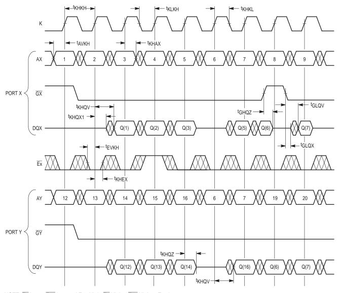
NOTE:  $\overline{Ex}$  Low =  $\overline{E1x}$  Low and E2x High.  $\overline{Ex}$  High =  $\overline{E1x}$  High or E2x Low.
