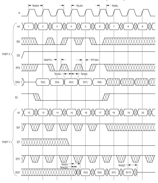
NOTES:  $\overline{Ex}$  Low =  $\overline{E1x}$  Low and E2x High.  $\overline{Ex}$  High =  $\overline{E1x}$  High or E2x Low.
