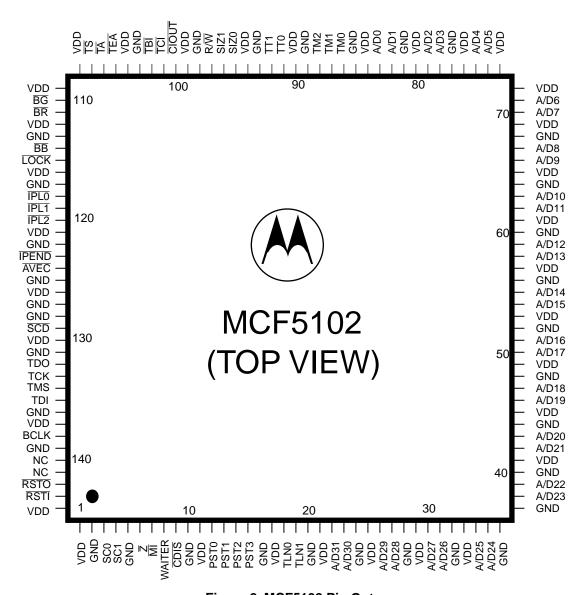
Figure 2. MCF5102 Pin Out
