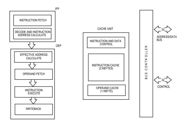
Figure 1. MCF5102 Block Diagram
