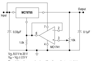
The addition of an operational amplifier allows adjustment to higher or intermediate values while retaining regulation characteristics. The minimum voltage obtainable with this arrangement is 3.0 V greater than the regulator voltage.
