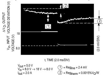
Figure 2. MC78T05AC Load and Thermal Regulation
