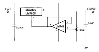
Figure 11. Adjustable Output Regulator (7 to 30V)
