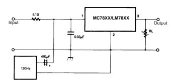
Figure 7. Ripple Rejection
