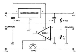
Figure 14. Tracking Voltage Regulator
