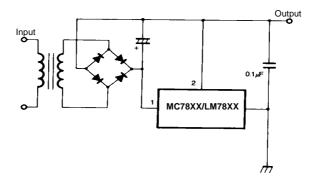
Figure 16. Negative Output Voltage Circuit
