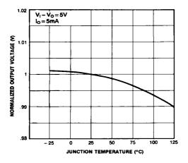
Figure 3. Output Voltage
