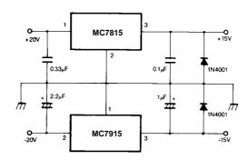
Figure 15. Split Power Supply (±15V-1A)
