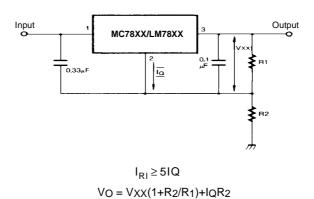
Figure 10. Circuit for Increasing Output Voltage
