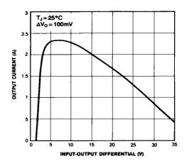
Figure 2. Peak Output Current
