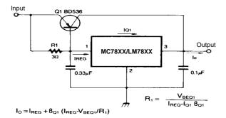
Figure 12. High Current Voltage Regulator
