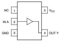
Figure 1. Pinout (Top View)
