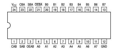
Figure 2. 24-Lead Pinout (Top View)
