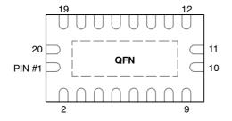
Figure 1. Pinouts: 20-Lead (Top View)
