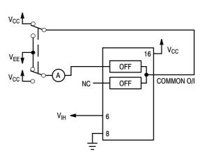
Figure 10. Maximum Off Channel Leakage Current, Any One Channel, Test Set-Up
