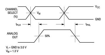
Figure 13. Propagation Delays, Channel Select to Analog Out
