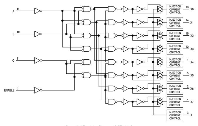
Figure 21. Function Diagram, HCT4851A
