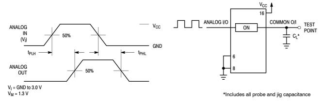
Figure 15. Propagation Delays, Analog In to Analog Out
