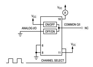
Figure 19. Power Dissipation Capacitance, Test Set-Up
