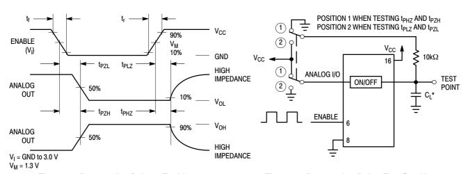
Figure 17. Propagation Delays, Enable to Analog Out
