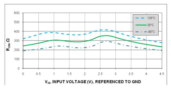
Figure 5. Typical On Resistance  $V_{CC} = 4.5V$
