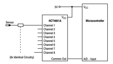
Figure 8. MC74HCT4851A Solution
