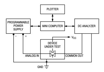
Figure 9. On Resistance Test Set-Up
