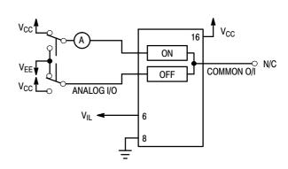
Figure 12. Maximum On Channel Leakage Current, Channel to Channel, Test Set-Up
