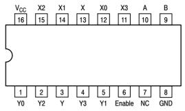
Figure 4. MC74HCT4852A 16-Lead Pinout (Top View)
