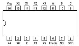
Figure 2. MC74HCT4851A 16-Lead Pinout (Top View)
