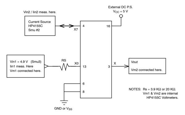
Figure 6. Injection Current Coupling Specification
