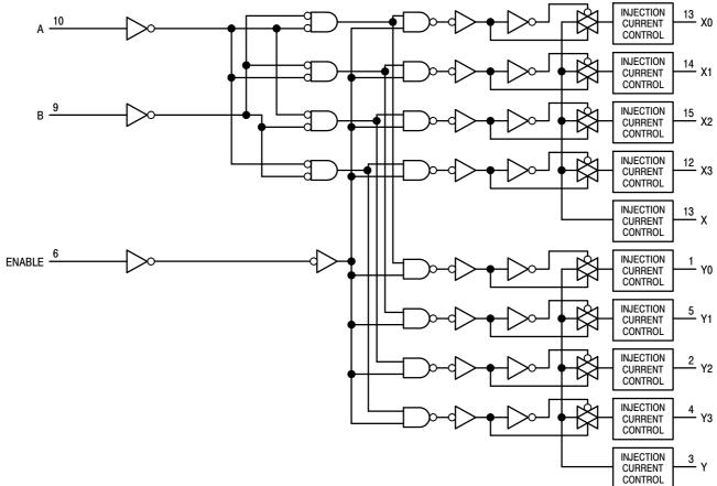
Figure 22. Function Diagram, HCT4852A
