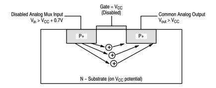
Figure 20. Diagram of Bipolar Coupling Mechanism
