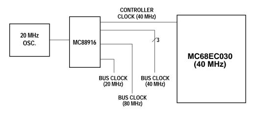
Figure 1. MC68EC030 Clock Circuitry
