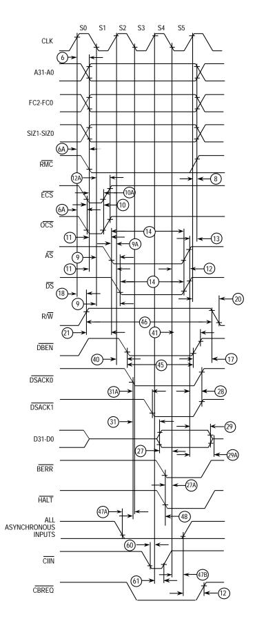
Figure 11. Asynchronous Read Cycle Timing Diagram
