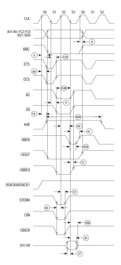
Figure 13. Synchronous Read Cycle Timing Diagram
