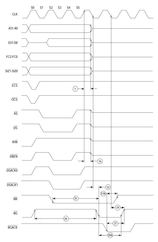
NOTE: Timing measurements are referenced to and from a low voltage of 0.8 V and a high voltage of 2.0 V, unless otherwise noted. The voltage swing through this range should start outside and pass through the range so that the rise or fall will be linear between 0.8 V and 2.0 V.
