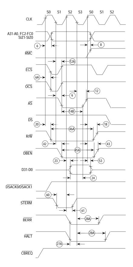
Figure 14. Synchronous Write Cycle Timing Diagram
