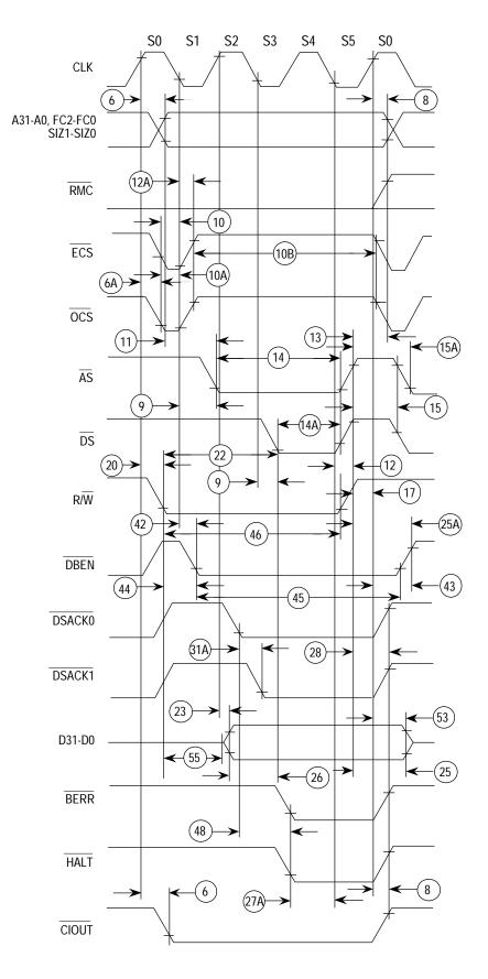
Figure 12. Asynchronous Write Cycle Timing Diagram
